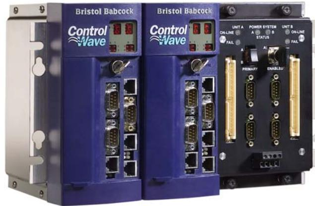
ControlWave Redundancy Systems include a stainless steel chassis that houses the primary and standby CPU's and Power Supply Modules. The chassis also houses the ControlWave CPU and Communications Redundancy Switch Module. The Switch Module allows automatic and manual selection of the primary controller CPU in case of hardware failure, and will additionally switch up to four serial communication ports to the selected primary CPU of the pair.
