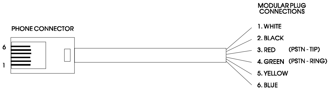
Figure 2-14 - Wiring for Phone Cord Connector
