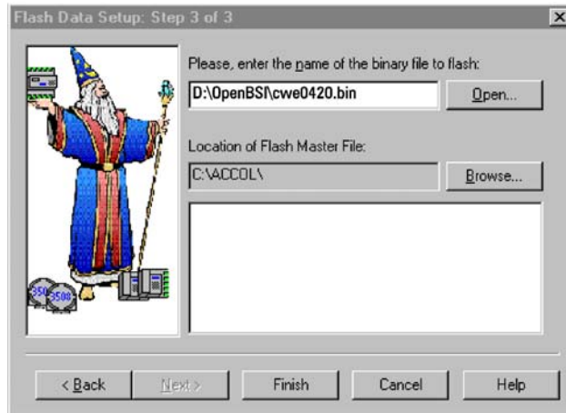
Figure 2-27 - Flash Data Setup Menu (Note: Substitute \cwi0420.bin for cwe04...)
